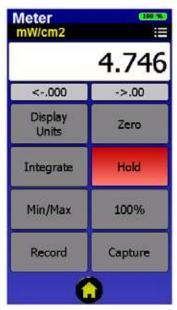
application for steady-state light measurements and includes features such as Integrate, Hold, Zero, Min/Max/Peak, as well as data recording all with the touch of a button. The screen can be viewed in both portrait (tall) and landscape (wide) modes.
