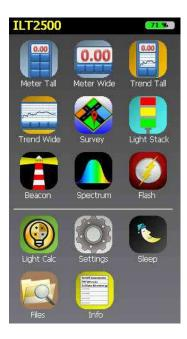
**Survey** allows data to be sorted by location or light source and **Light Stack** has a programmable color changing display (red/yellow/green) and sound alert for quick troubleshooting.
